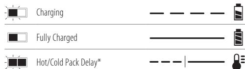
\*The red light will continue to blink, but a yellow indicator light will be illuminated during this operation. Once the battery pack has reached an appropriate temperature, the yellow light will turn off and the charger will resume the charging procedure.
